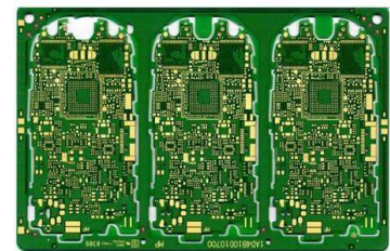
6-Layer ENIG PCB material:FR4 Borad thickness:1.8mm copper thickness:1oz panel size: 194.86mm*136.20mm(3pcs)
