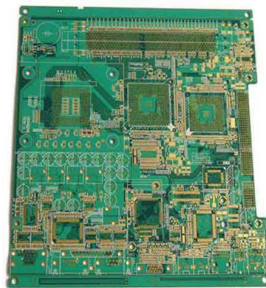
16-layer OSP PCB material:FR4 Borad thickness:2.5mm copper thickness:2oz size: 232.52mm*165.80mm
