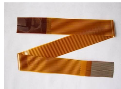
1-Layer FPC material:PI Borad thickness:0.08mm copper thickness:0.5oz size: 300.08mm*19.50mm
