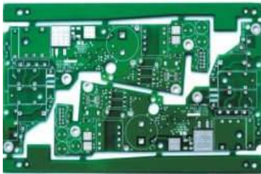
2-Layer Lead free HASL PCB material:Taconic Borad thickness:1.6mm copper thickness:1oz panel size: 208.52mm*136.20mm(2pcs)
